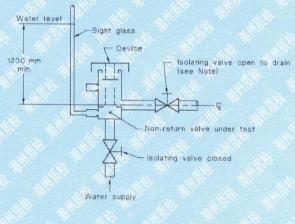
NOTE: To be within ±10 mm of valve under test.
